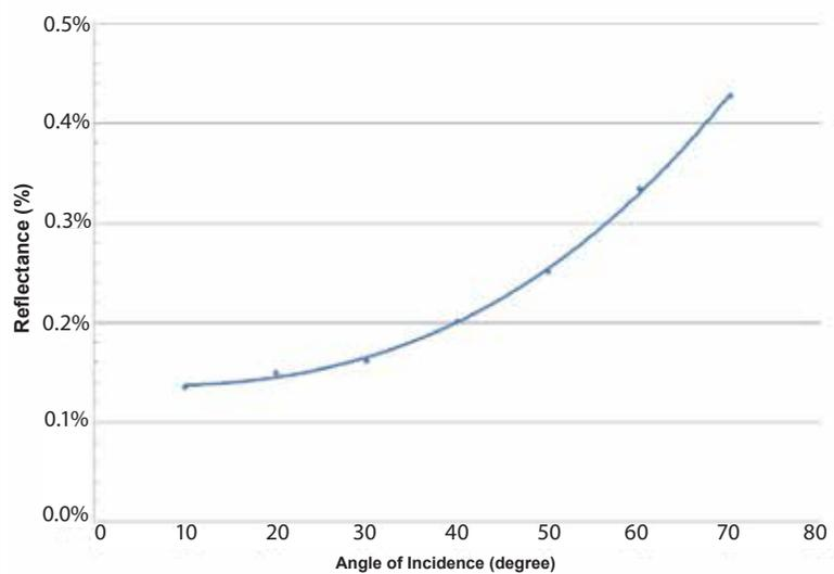
VANTABLACK®S-IR exhibits low reflectance (<1%) as a function of incident angle of illumination. This property is important for stray light control and cold shield design performance.
