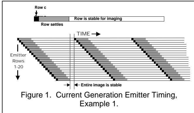
some delay between the last row change and the start of the next frame at the first row. If a higher frame rate is required this delay can be reduced, resulting in the system timing of Figure 2.
