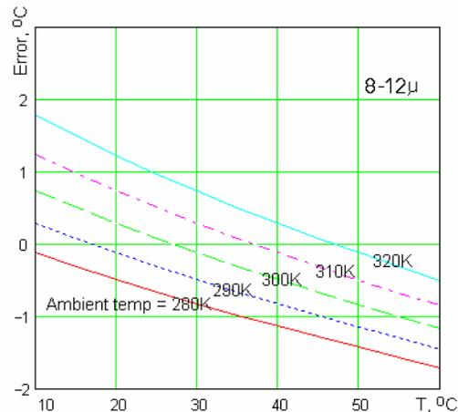
Some commercial blackbodies attempt to compensate for radiometric losses by inserting a gain or offset correction into the temperature setpoint. But the ambient temperature dependence and wavelength
