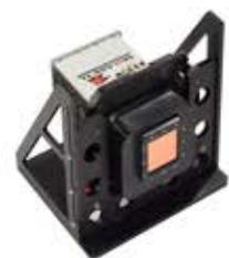
The DEE is an advanced micro-emitter array. This state-of-the-art integrated circuit is constructed of thermally isolated mechanical structures with deposited thin film resistive heaters, fabricated on an advanced sub-micron silicon read-in integrated circuit (RIIC).
