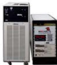
The TSS includes power supplies, refrigerated chiller, an ion pump controller for DEE operation and a top-level ICD. Custom length cables and hoses available.
