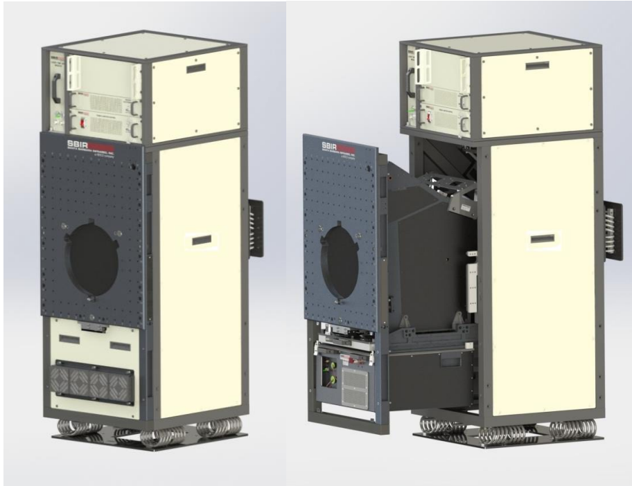
Figure 1 – Future E-O (FEO) TMDE System. Standard operating configuration (left) and target projector access configuration (right) shown.
